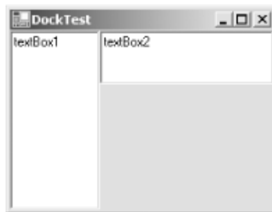
Figure 5-11. Docking two controls to adjacent sides of a form
