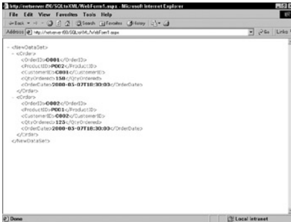
Figure 13-4: Output of the application that converts relational data into an XML document
